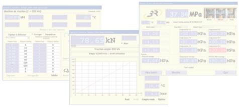
Thanks to the touch screen, the operator can select the jack and launch each test of the batch. At the end, the average value is automatically calculated following the request of EN standard and all results are sent to a custom report.
