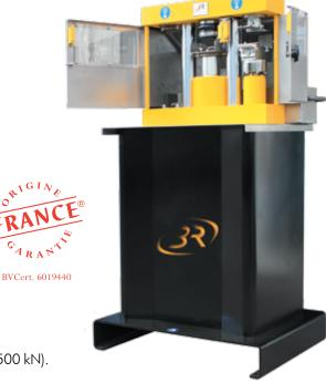
Our standard testing machine is equipped with 2 jacks: 1 for flexural tests (max load from 8 to 50 kN) and 1 for compressive tests (max load from 200 to 500 kN). **Option:** 3rd jack for low range compressive tests (see above picture). Once again, great care has been given to ergonomics, with high pedestral, transparent doors, crumb collector and so on.
